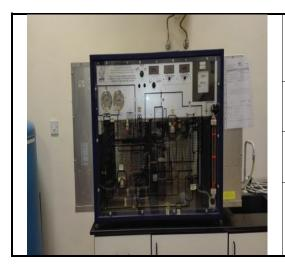
**Device Name:** Air conditioning study unit and reversing cycle heat pump with double evaporator.
