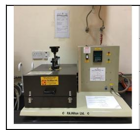
**Device Name:** The thermal conductivity of building and insulating materials unit
