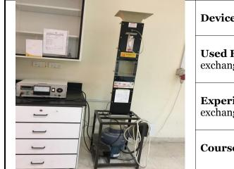
**Device Name:** Cross flow heat exchanger apparatus
